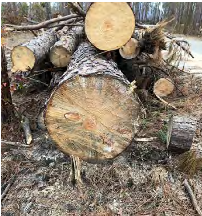
Figure 31. Stacked pine logs showing blue stain.
